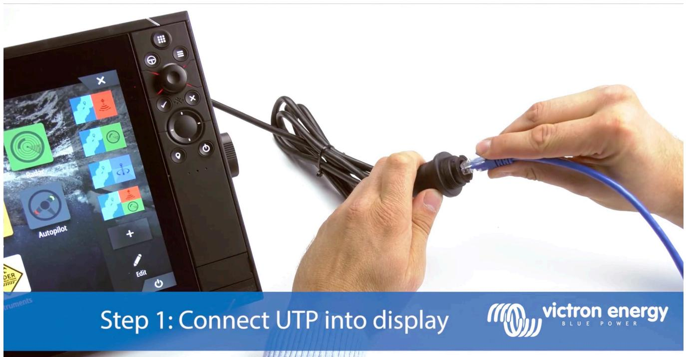
Step 1: Connect UTP into display
