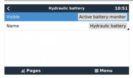
No other settings, such as IP addresses or similar are required. The GX device and the Navico devices connect to each other using a technology called linklocal addressing.
