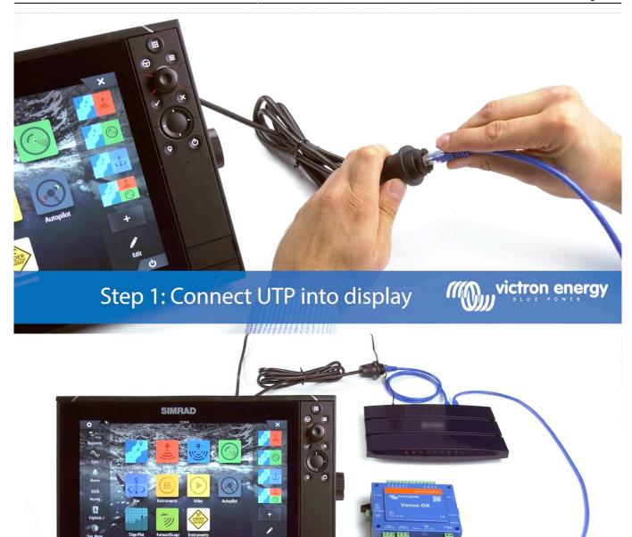
Step 2: connect UTP cable into Victron Venus GX, Color Control GX or Octo GX
