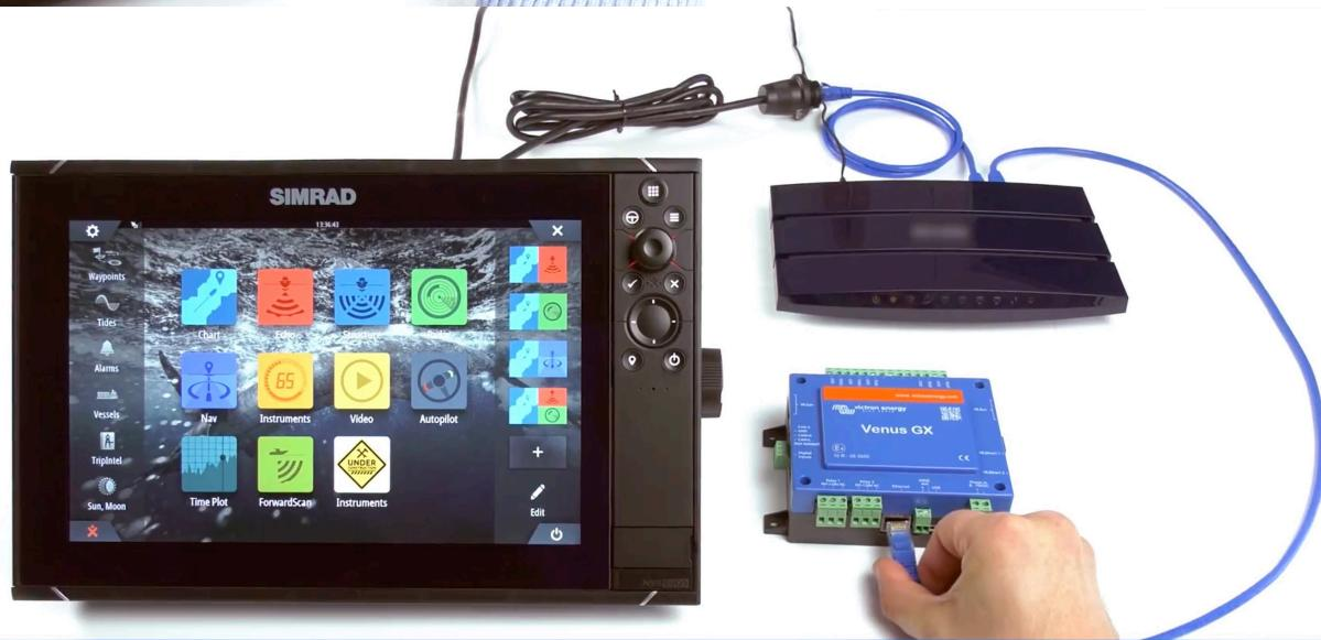
Step 2: connect UTP cable into Victron Venus GX, Color Control GX or Octo GX
