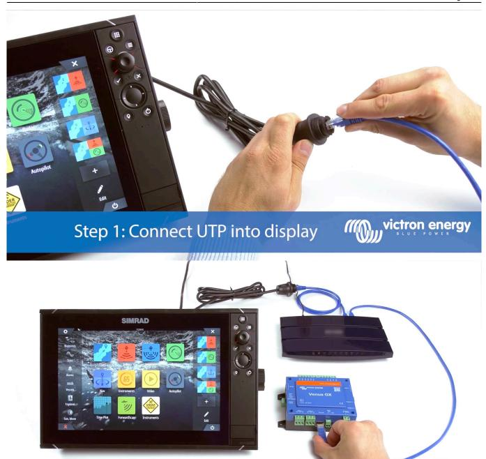
Step 2: connect UTP cable into Victron Venus GX, Color Control GX or Octo GX
