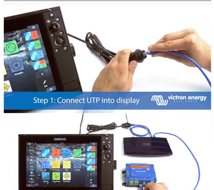
Step 2: connect UTP cable into Victron Venus GX, Color Control GX or Octo GX
