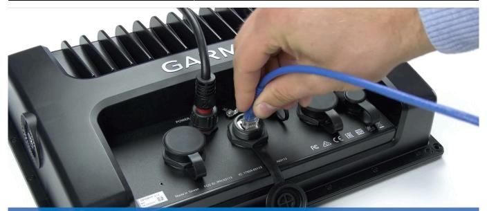
Step 1: Connect UTP into display
