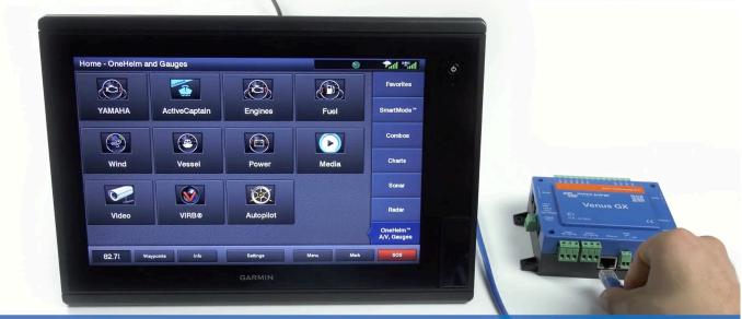
Step 2: connect UTP cable into Victron
