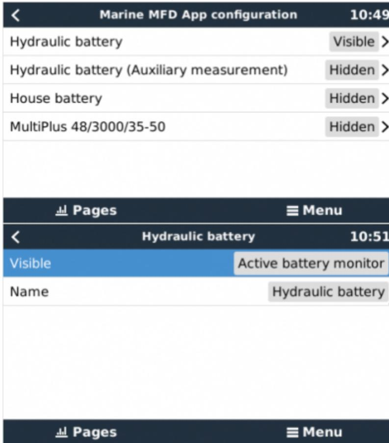
3. For boats; and other applications with DC loads such as lighting and a Battery Monitor installed, make sure to enable the "Has DC system setting". For more information about it; see the [GX Manual](#).
