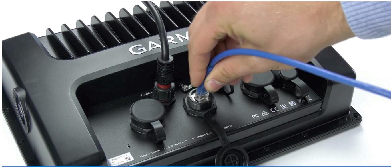
Step 1: Connect UTP into display
