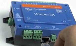
Step 2: connect UTP cable into Victron
