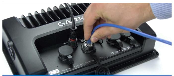
Step 1: Connect UTP into display
