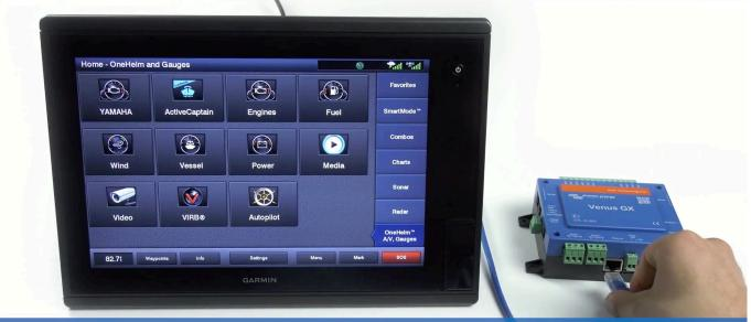
Step 2: connect UTP cable into Victron
