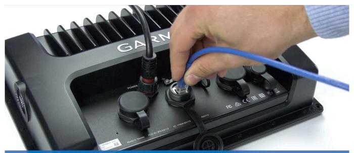
Step 1: Connect UTP into display
