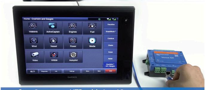
Step 2: connect UTP cable into Victron
