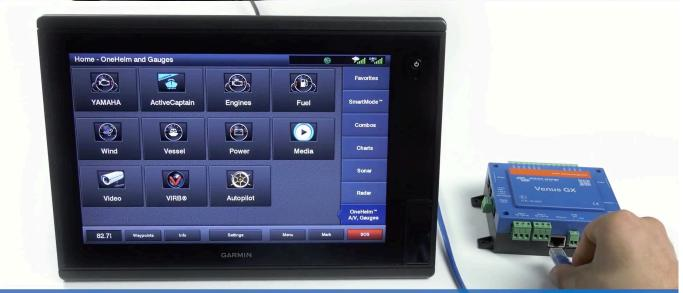
Step 2: connect UTP cable into Victron
