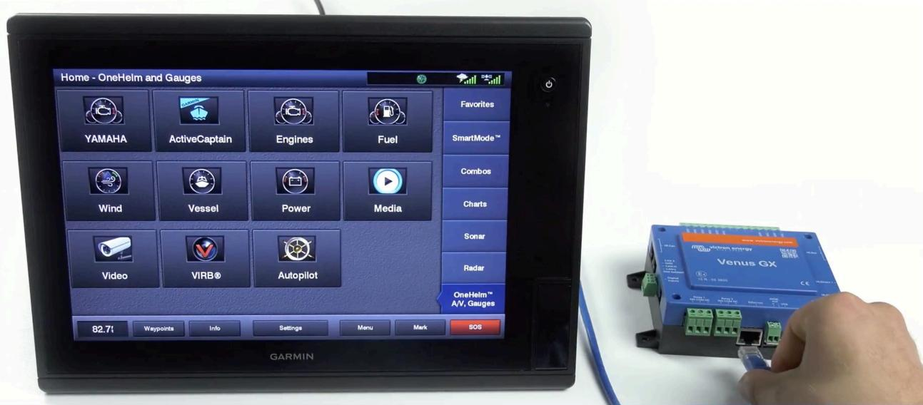
Step 2: connect UTP cable into Victron Venus GX, Color Control GX or Octo GX
