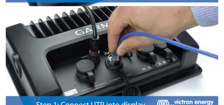
Step 1: Connect UTP into display
