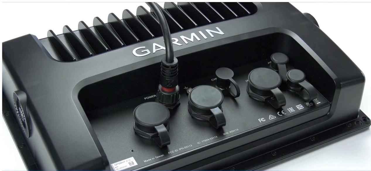
Step 1: Connect UTP into display
