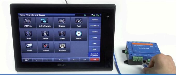
Step 2: connect UTP cable into Victron
