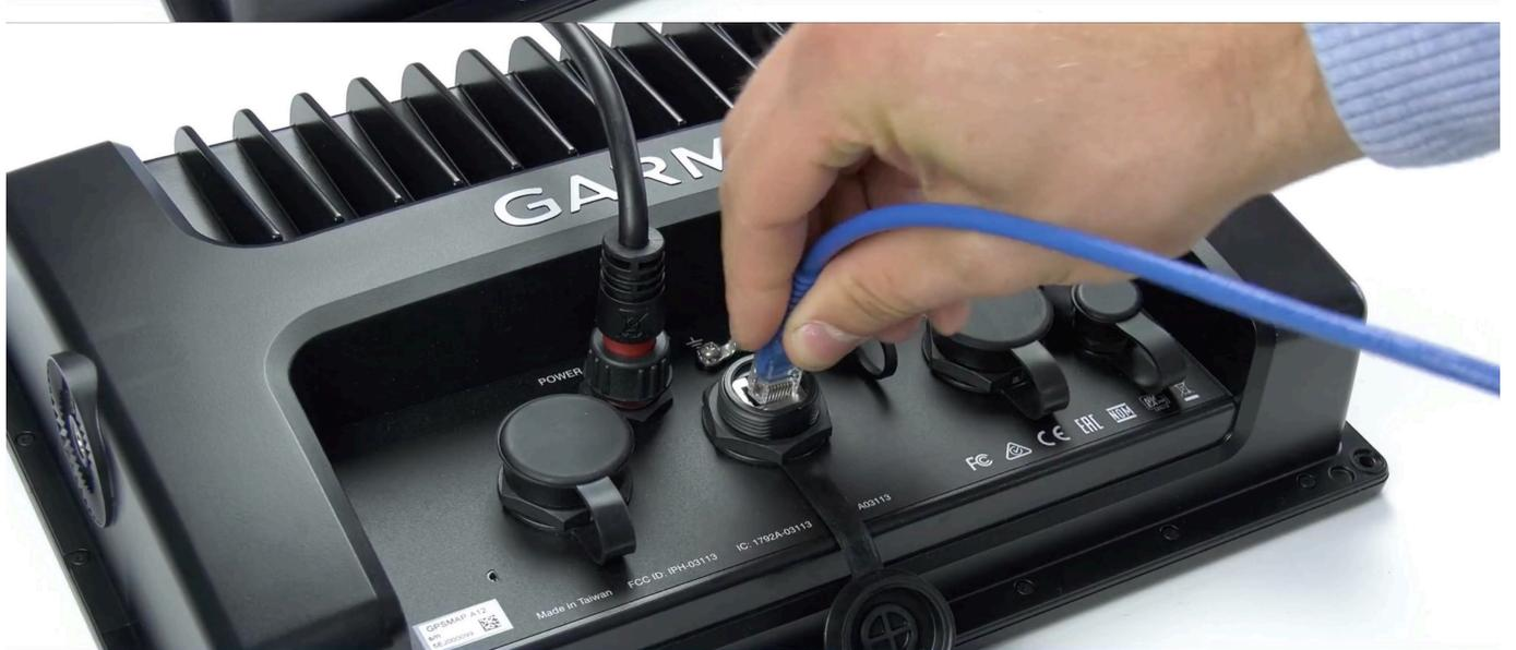
Step 1: Connect UTP into display
