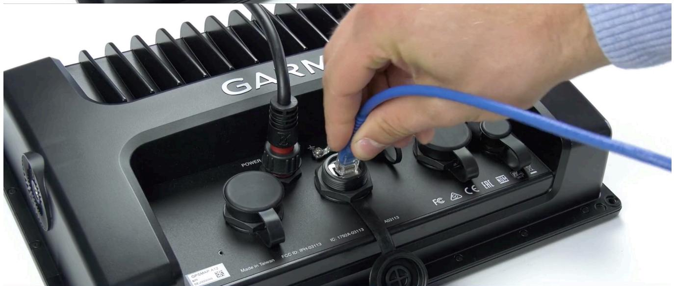
Step 1: Connect UTP into display
