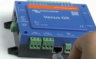
Step 2: connect UTP cable into Victron Venus GX, Color Control GX or Octo GX
