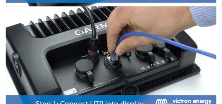
Step 1: Connect UTP into display
