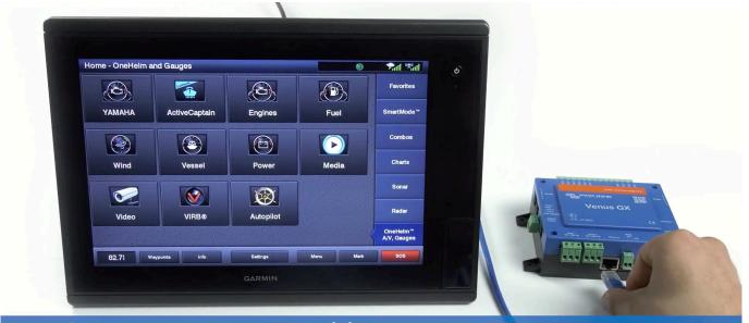
Step 2: connect UTP cable into Victron
