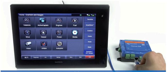
Step 2: connect UTP cable into Victron
