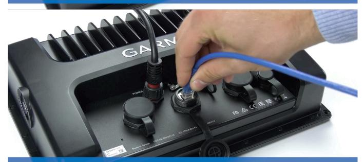
Step 1: Connect UTP into display
