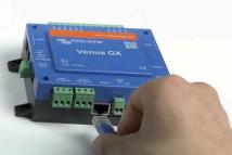
Step 2: connect UTP cable into Victron
