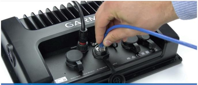
Step 1: Connect UTP into display
