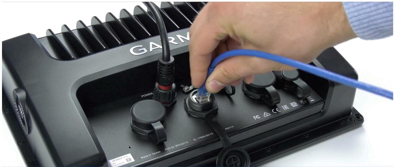
Step 1: Connect UTP into display
