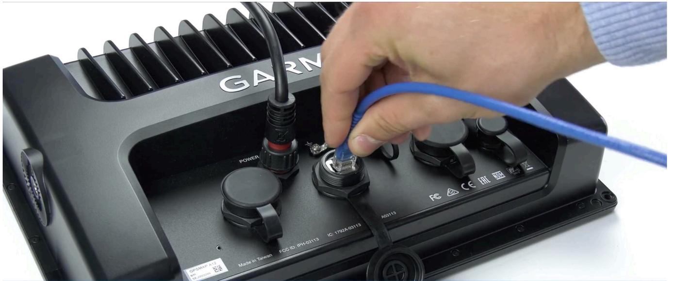
Step 1: Connect UTP into display
