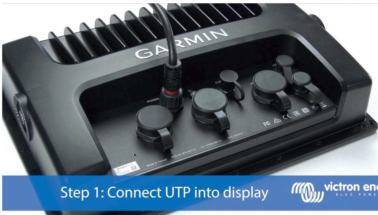
Step 1: Connect UTP into display
