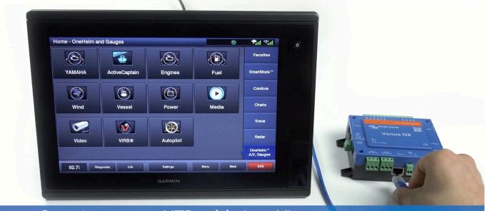
Step 2: connect UTP cable into Victron Venus GX, Color Control GX or Octo GX victron energy
