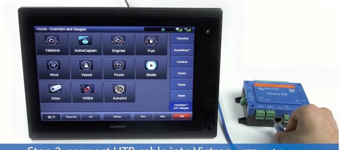
Step 2: connect UTP cable into Victron
