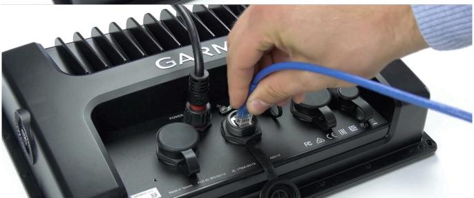
Step 1: Connect UTP into display
