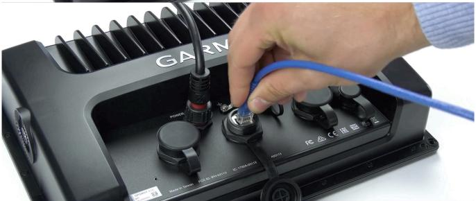
Step 1: Connect UTP into display
