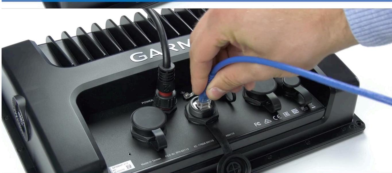
Step 1: Connect UTP into display
