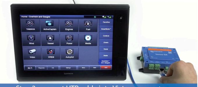
Step 2: connect UTP cable into Victron
