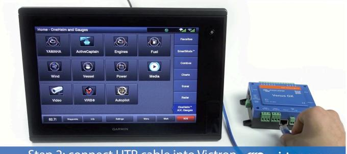
Step 2: connect UTP cable into Victron
