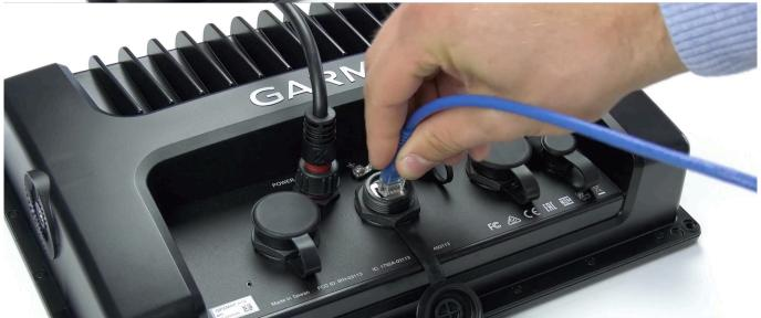
Step 1: Connect UTP into display
