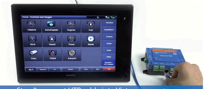
Step 2: connect UTP cable into Victron
