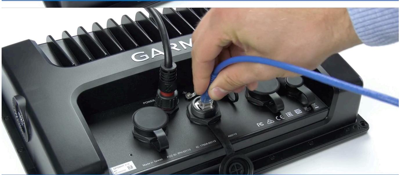
Step 1: Connect UTP into display
