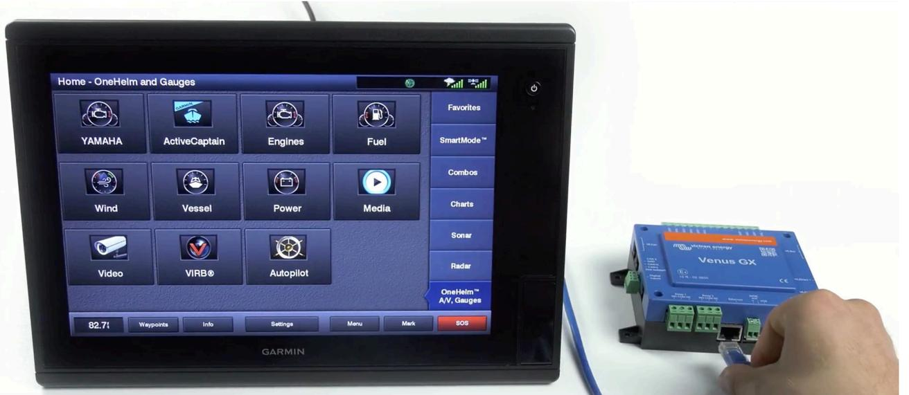
Step 2: connect UTP cable into Victron Venus GX, Color Control GX or Octo GX
