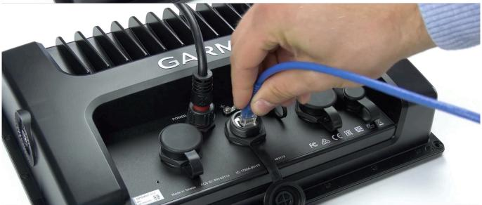
Step 1: Connect UTP into display
