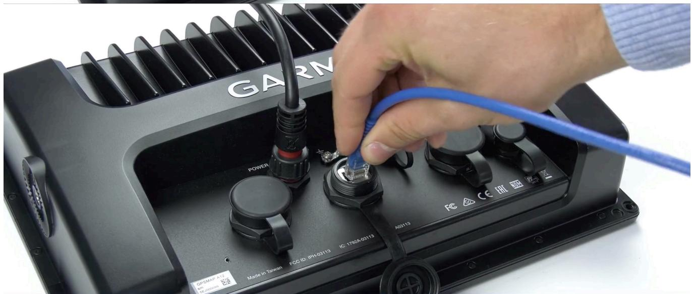
Step 1: Connect UTP into display
