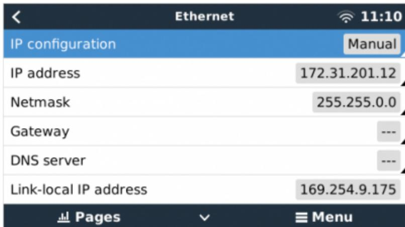
It is possible to connect a router to the same LAN; and that way connect the GX Device to the internet. Make sure the *Gateway* and *DNS Server* settings of the GX are set to the IP address of the router, and that the router has its LAN IP addressing configured in the same subnet.
