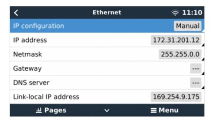
It is possible to connect a router to the same LAN; and that way connect the GX Device to the internet. Make sure the *Gateway* and *DNS Server* settings of the GX are set to the IP address of the router, and that the router has its LAN IP addressing configured in the same subnet.
