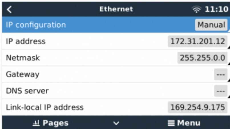
It is possible to connect a router to the same LAN; and that way connect the GX Device to the internet. Make sure the *Gateway* and *DNS Server* settings of the GX are set to the IP address of the router.
