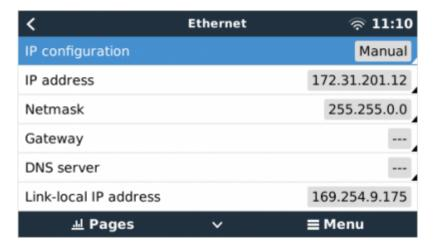
It is possible to connect a router to the same LAN; and that way connect the GX Device to the internet. Make sure the *Gateway* and *DNS Server* settings of the GX are set to the IP address of the router.
