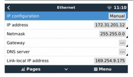
It is possible to connect the a router to the same LAN; and that way connect the GX Device to the internet. Make sure the *Gateway* setting of the GX is set to the IP address of the router.
