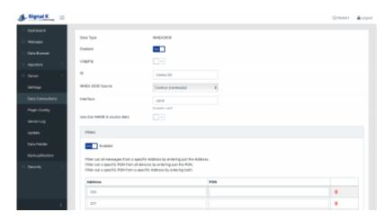
Note that, to keep that operational, that port must be configured as a 250kbit VE.Can & NMEA2000 port in the Remote Console.
