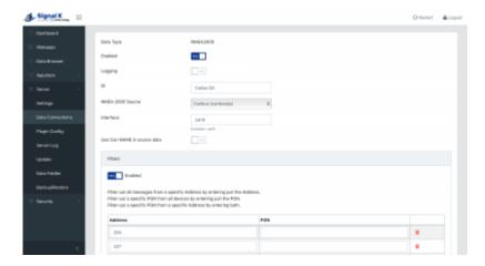
Note that, to keep that operational, that port must be configured as a 250kbit VE.Can & NMEA2000 port in the Remote Console.
