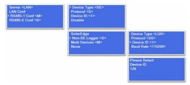
Once you are done with the SunSpec setup you can re-configure RS485-1 for your SolarEdge Grid meter. The SolarEdge meter is still required for a zero export setup. The SunSpec setting will remain in the memory of the SolarEdge.
