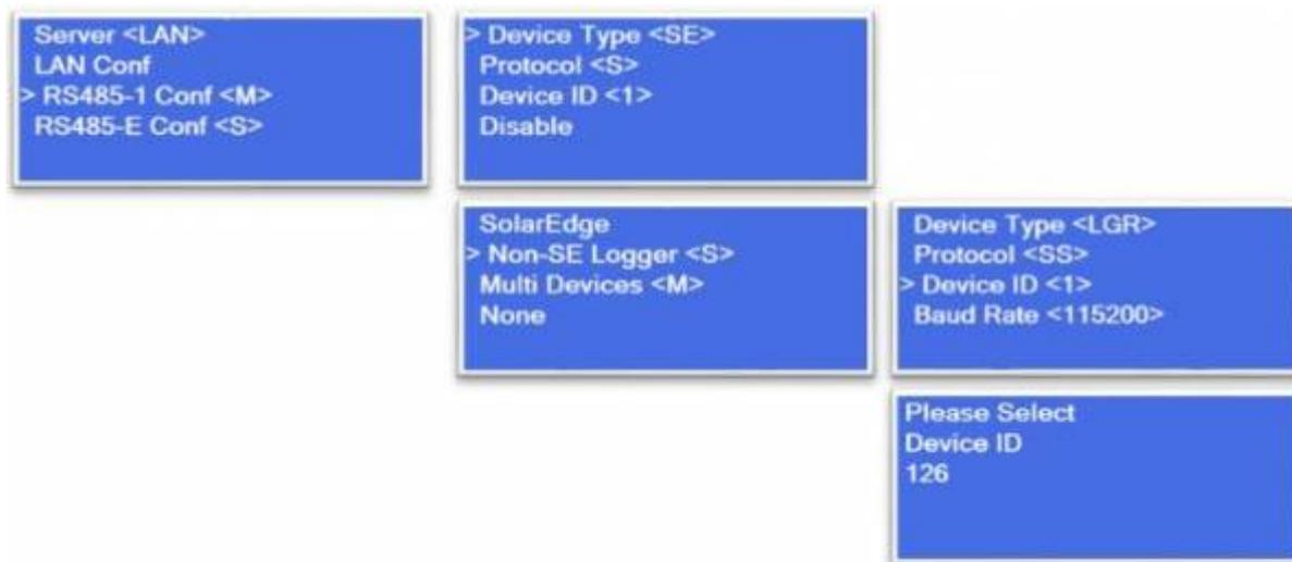
Once you are done with the SunSpec setup you can re-configure RS485-1 for your SolarEdge Grid meter. The SolarEdge meter is still required for a zero export setup. The SunSpec setting will remain in the memory of the SolarEdge.
