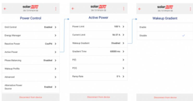
Inverters with LCD • Power Control □ Active Power control □ Wakeup Gradie □ Disable
