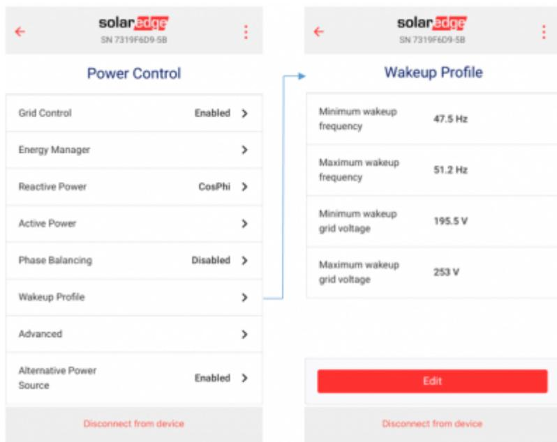
Inverters with LCD: • Power Control □ Wakeup Profile □ Edit
