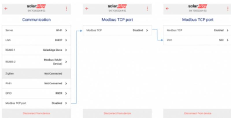
Inverters with LCD • Communication □ LAN Conf □ Modbus TCP □ TCP Port □ Edit port to 502
