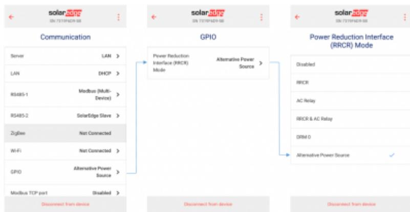
Inverters with LCD • Enter the inverter’s setup menu using the SolarEdge Password. • Communication □ GPIO Conf □ Device Type □ Alternative Power Src.
