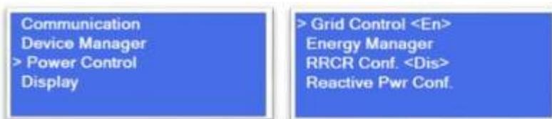
2. Configure Wakeup Conf. • Power Control □ Wakeup Profile □ Edit • Edit Maximum Wake up Frequency = 51.2Hz
