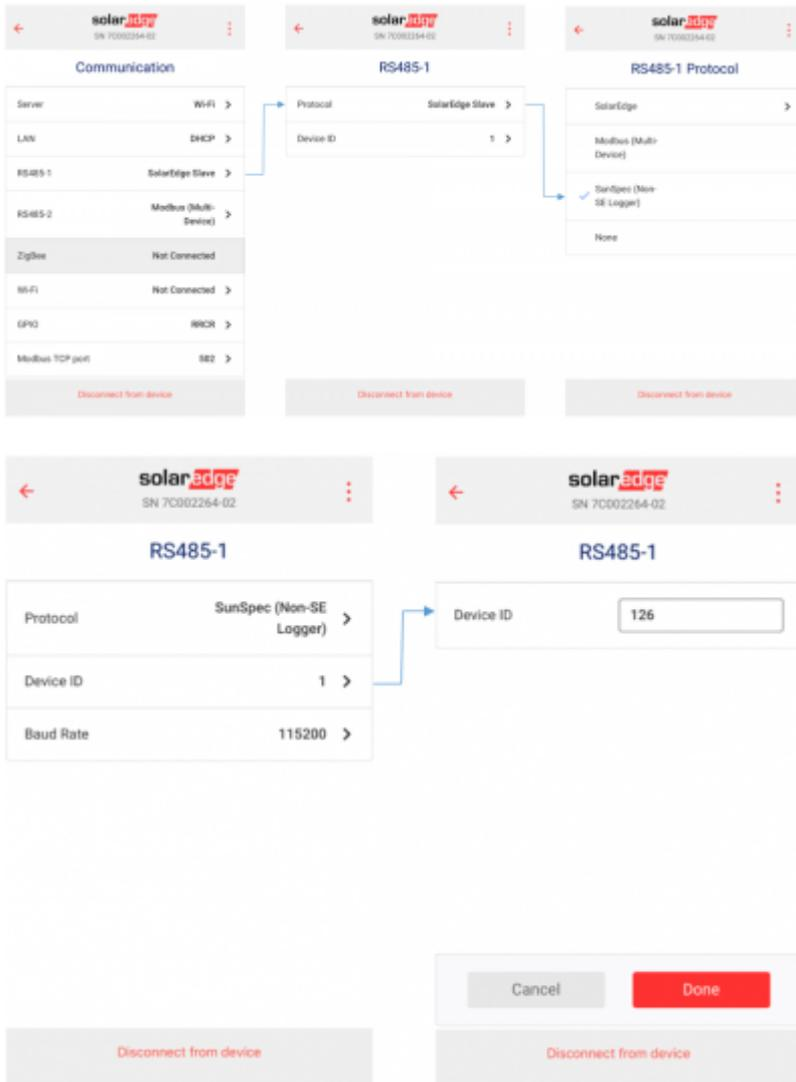
Inverters with LCD • Communication □ RS481 □ Device Type □ Non-SE Logger □ Device ID □ Edit to 126
