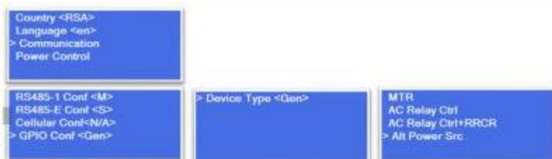
3. How to configure Frequency Shifting Important note: Please ensure the SolarEdge inverter and your VE.Bus Config is setup for the same frequency bandwidth. For systems that can feed back into the grid or for pure off-grid systems: 1. Enable frequency shifting • Go into Power Control • Ensure Grid control is Enabled
