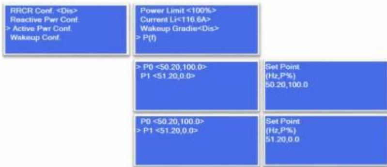
For systems with zero grid feed-in In addition to the frequency settings above, please set the following: 1. Configure P(f) for APS • Power Control □ Alternative Power Source □ P(f) • Edit P0: 50.5Hz, 100% Power • and P1: 51.2Hz, 0% Power
