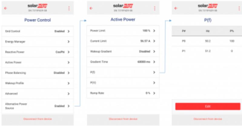
Inverters with LCD • Power Control □ Active Power control □ P(f) • Edit P0: 50.5Hz, 100% Power • and P1: 51.2Hz, 0% Power
