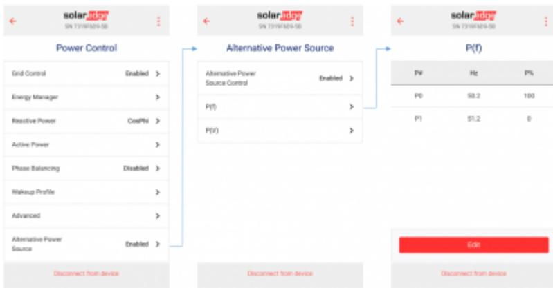
Inverters with LCD • Power Control □ Alt Power Src□ P(f) • Edit P0: 50.5Hz, 100% Power • and P1: 51.2Hz, 0% Power
