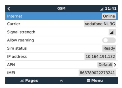
When using a SIM card with its SIM-pin security disabled, the system will work without further configuration.
