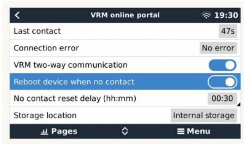
Note that if you are leaving internet service coverage areas (such as an RV on the move, or a boat leaving dock to go to sea) then it is recommended to disable this setting, so that your GX is not rebooting itself for no reason. Or set it, for example, to a two hour time-out. And accept a reboot every two hours when underway.
