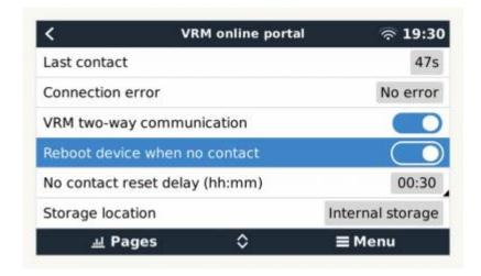
Note that if you are leaving internet service coverage areas (such as an RV on the move, or a boat leaving dock to go to sea) then it is recommend to disable this setting, so that your GX is not rebooting itself for no reason. Or set it, for example, to a two hour time-out. And accept a reboot every two hours when underway.
