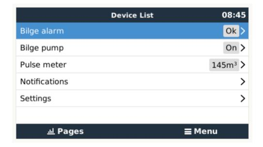
Other parameters related to that function can be configured by entering the device menu and selecting Setup. For pulse meters, you can configure the unit, the multiplier (the volume represented by each pulse) and reset the counter.
