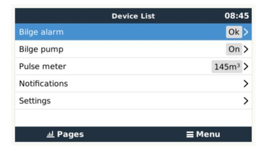
Other parameters related to that function can be configured by entering the device menu and selecting Setup. For pulse meters, you can configure the unit, the multiplier (the volume represented by each pulse) and reset the counter.
