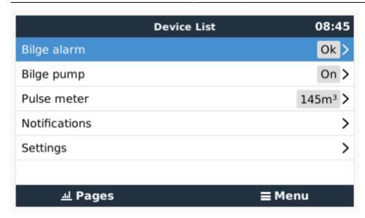
Other parameters related to that function can be configured by entering the device menu and selecting Setup. For pulse meters, you can configure the unit, the multiplier (the volume represented by each pulse) and reset the counter.
