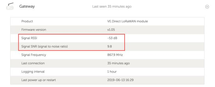
A higher RSSI (Received Signal Strength Indicator) indicates a better signal, where -30dB is the best possible, and -130 dB the worst: no signal it all. Everything below -75 dB is considered a bad connection and has a high risk of packet loss. The SNR is the Signal to Noise Ratio. This ranges from positive plus 10 to negative -20. Anything above 6 and below -10 is good.
