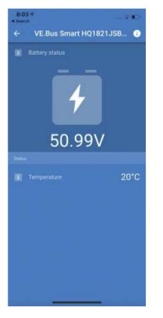
It takes a bit of time before a Multi is detected. When the dongle detects a Multi, *VictonConnect* will identify the Multi in the Device list. Shortly after updating the firmware in *VictronConnect* only the dongle will show up in the device list. If connected, a re-scan will reveal the *Multi*.
