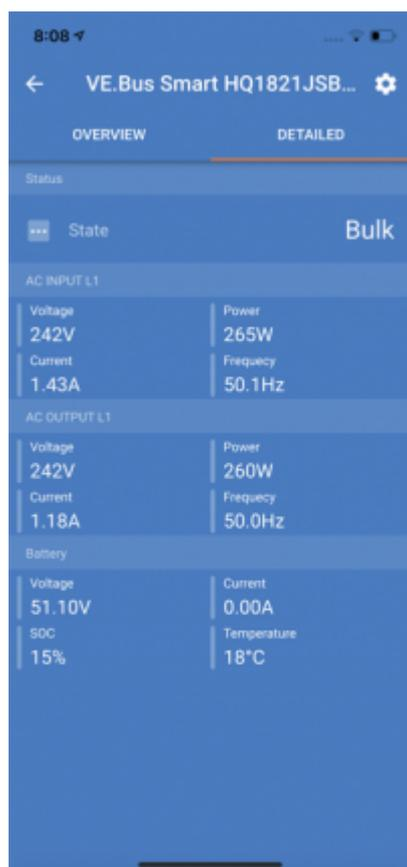
When used with Multi- inverter/chargers the dongle provides *on-battery* temperature and voltage sensing capabilities - allowing compensation for possible cable losses which can occur during charging and discharging. Temperature sensing allows accurate temperature-compensation during battery charge cycles. On MultiPlus-II models the dongle is, at present, the *only* way to add an “on-battery” sensing capability.
