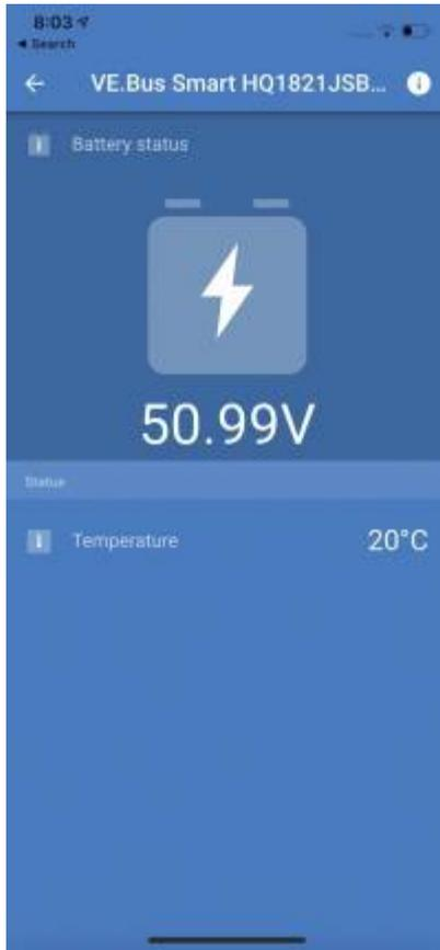
It takes a bit of time before a Multi is detected. When the dongle detects a Multi, *VictronConnect* will identify the Multi in the Device list. Shortly after updating the firmware in *VictronConnect* only the dongle will show up in the device list. If connected, a re-scan will reveal the *Multi*.
