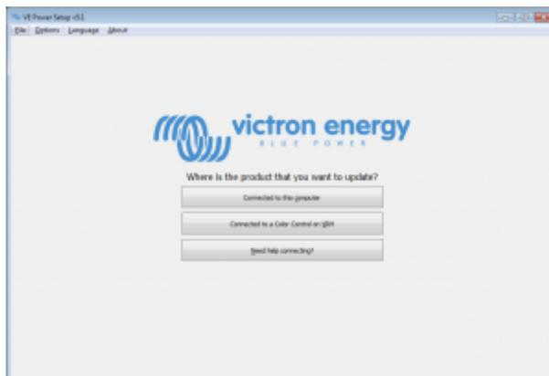
VE Power Setup is a tool to update firmwares locally and remotely, or to remotely perform VE Configure, in conjunction with VEConfig.
