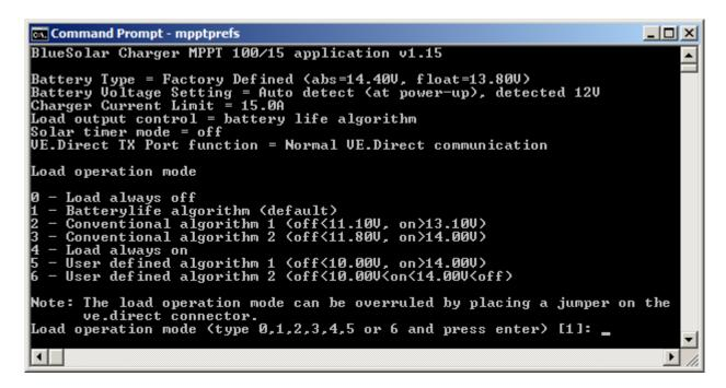
**h** - Modify load switch high voltage level (load operation modes 5 and 6)
