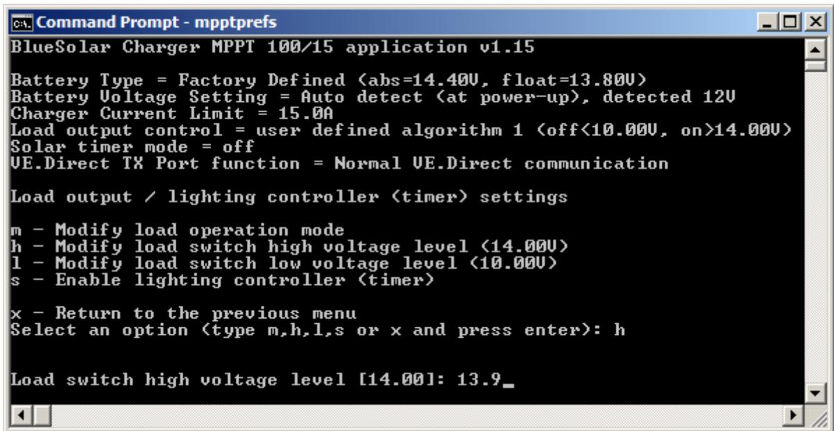
**l** - Modify load switch low voltage level (load operation modes 5 and 6)
