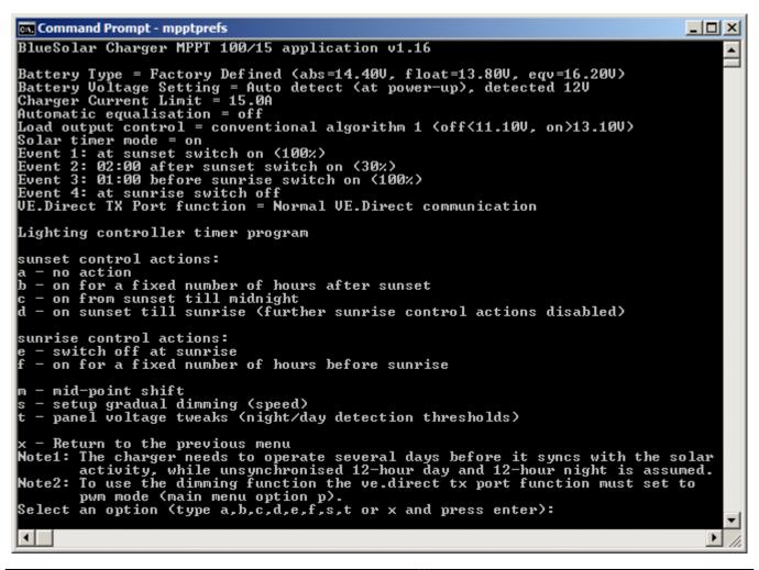
When the lighting controller is enabled (option 's'), a timer program can be created. The events 'sunset' and 'sunrise' are used as anchor points for the timer program. The lighting controller (timer) program is written to non-volatile memory, so the program will remain intact when the charger is disconnected from the battery.
