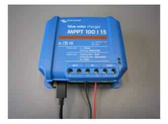
After successfully connecting the charger to the computer, there are two ways to change the settings. The common way is the interactive mode. When a large number of chargers must be (re)programmed, it might be useful to use the tool in batch mode. Both modes are explained:
