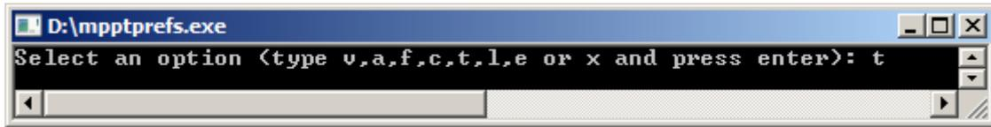
Note for models with a rotary switch: creating a user defined battery effectively disables the rotary switch. Use option 't' to enable the rotary switch again, and make the charge use the battery type as selected by the rotary switch position. Firmware version 1.15 has an improvement, changing the setting of the rotary switch will automatically enable it again.
