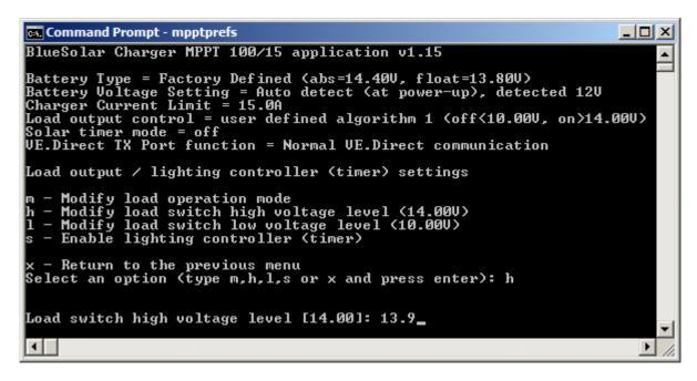
I - Modify load switch low voltage level (load operation modes 5 and 6)
