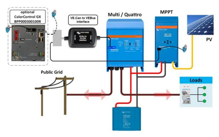
Either way, with or without CCGX, make sure that the VE.Can network is terminated on both sides, using the VE.Can terminators supplied with the CCGX and the MPPT charger controllers. They are also available for purchase as a separate accessory.
