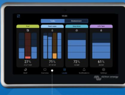
The view will automatically group tanks of the same type in case the system has so many tanks that they don't all fit on the screen individually.
