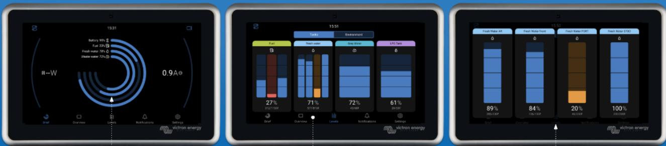
The total tank levels are displayed on the Brief view, which is particularly useful for systems with multiple tanks of the same type.
