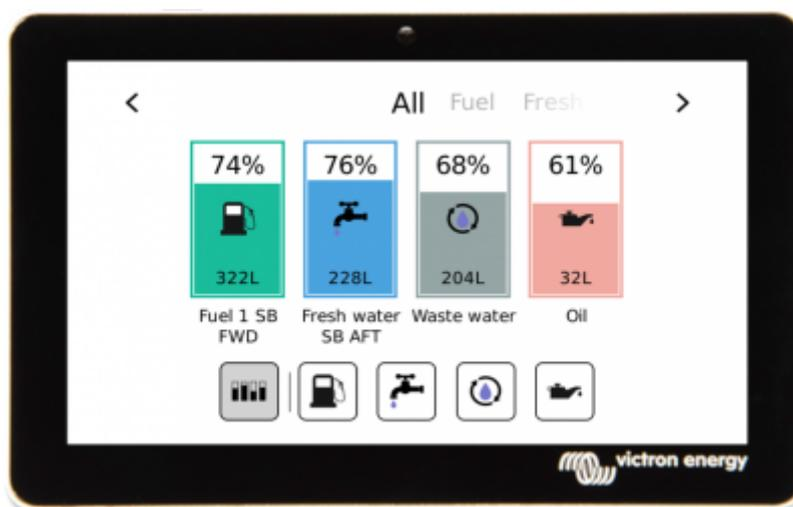
Above picture: GX Touch 50, showing multiple tank levels. Coming from either the NMEA2000
