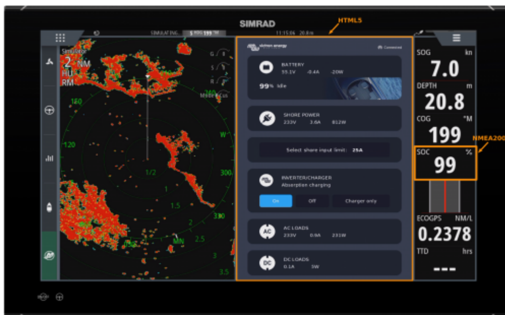
Picture showing the two integration options, NMEA2000 and HTML5 App. Click to see full size and see the difference between the two.
