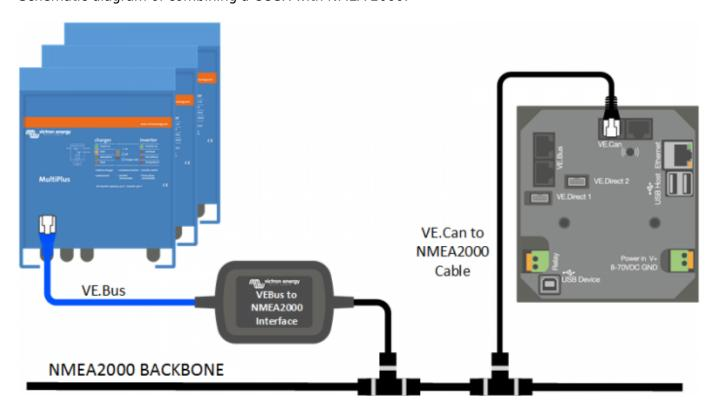
In above example, there needs to be a fuse in the VE.Can to NMEA2000 cable. Without it, the VE.Can
