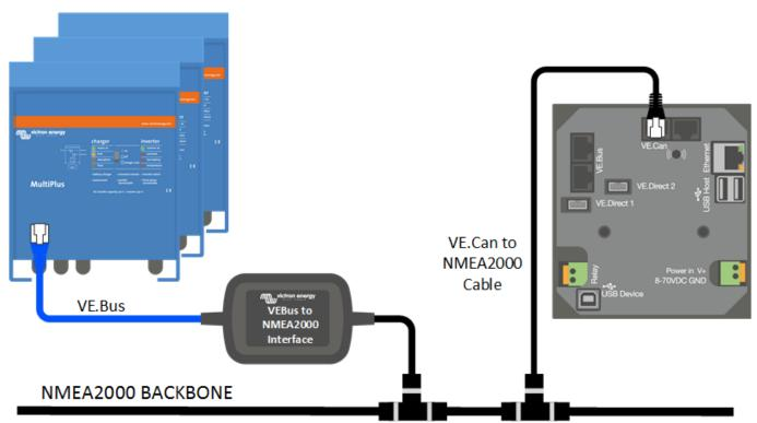
In above example, there needs to be a fuse in the VE.Can to NMEA 2000 cable. Without it, the VE.Can port in the CCGX will be left without power and therefore does not work.
