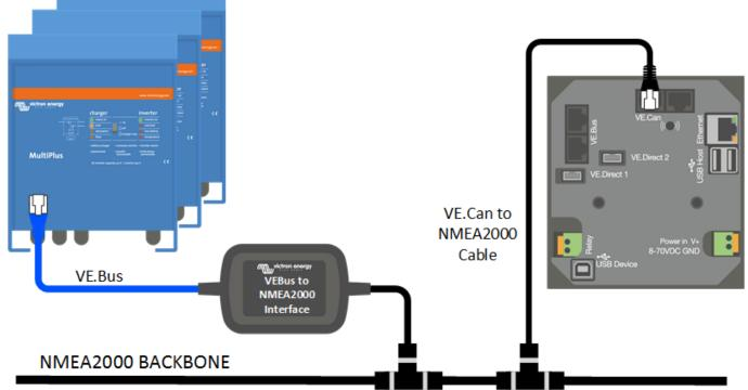
In above example, there needs to be a fuse in the VE.Can to NMEA 2000 cable. Without it, the VE.Can port in the CCGX will be left without power and therefore does not work.
