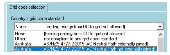
After configuration, always confirm that the system is safe with routine electrical safety checks in both modes (eg test RCD operation with AC input connected and disconnected).
