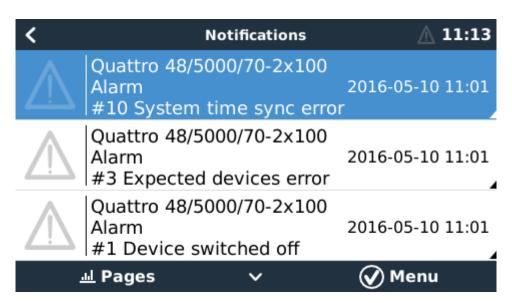
The real problem is Error 1. In this example it was caused by switching device L2 off with the front toggle switch. It was then quickly followed by Error 3. And when switching device L2 back on, briefly Error 10 is visible, followed by full recovery.
